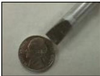
The standard tip size that comes with an iron is usually from 1/4" to 3/8" wide. This size works well for soldering either copper foil or lead came projects.
