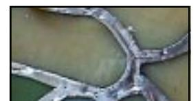
"Tin" the entire perimeter making sure to work some solder into seams that intersect the perimeter. (Tinning is the process of coating a surface with a thin layer of solder. Apply just enough solder to turn the foil to the silver color of the solder.) This creates a "dam" that prevents solder from spilling over the edge when you solder the interior seams.
