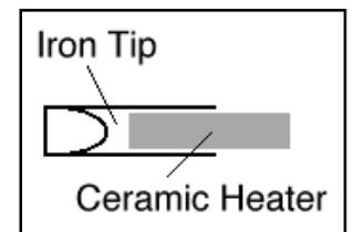
A remarkable feature of ceramic heater irons is they generally reach operating temperature in less than 60 seconds. Of the three types of nonconventional irons, the ceramic heater type best maintains consistent tip temperature over extended periods of time. Problems with slow heat recovery generally don't exist. A ceramic heater iron offers excellent flexibility and can be used with a temperature controller if you like.
