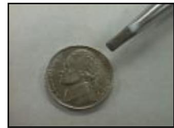
Very small tips, 1/8" or narrower, are usually used for decorative soldering. They allow you to create very fine details and designs with the solder.
