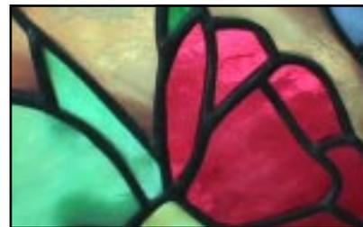
**50/50 Solder:** This is composed of 50% tin and 50% lead. It is liquid at 421°F, solid at 361°F and has a pasty range of 60 degrees. This solder will produce a much "flatter" bead than 60/40. Because of its higher melting point, 50/50 solder is often used on the back (or inside) of a stained glass project to protect against "melt through" when soldering the front. Because it spreads and flattens out, 50/50 solder is often used when soldering lead came joints.
