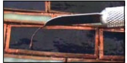
Set aside enough time to solder your entire project all at once. If you don't, dried flux and solder residues on the unfinished parts will make further soldering difficult. Flux allowed to remain on a project can compromise the strength of the solder joints.
