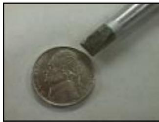
A smaller chisel tip, 3/16" wide, can be useful when soldering small pieces or when soldering in a tight area, such as a narrow inside part of a kaleidoscope. It is also very effective for decorative soldering.
