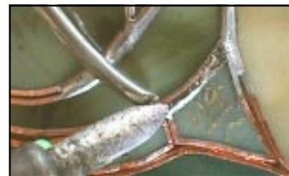
If you apply too little solder or move too quickly, your seam will be flat. To correct this problem, allow the solder to cool, then resolder the joint applying more solder. On the other hand, be careful not to feed the solder too fast or move the iron too slowly, as this will cause the solder seam to bulge and flow out over the glass.
