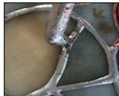
When you solder, work slowly enough to produce a good bead, but not so slowly that solder melts through seams to the back side of the project. Here's a hint: one way to prevent this is to put damp paper towel under your panel before you start soldering. Moving too slow also increases the likelihood of causing heat fractures on your glass.
