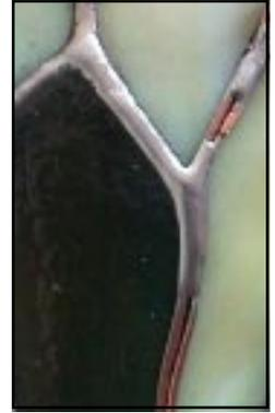
Avoid a "painting" motion when soldering. Visualize your iron as a magnet pulling along a metal strip. Maintain a small puddle of solder at the base of the tip as you solder. When two adjacent pieces of glass vary in thickness, ride the tip on the higher piece of glass as you solder.
